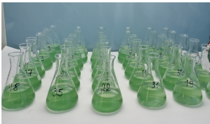
Figure 1. Erlenmeyer flasks with the inoculated culture of Spirulina platensis on Zarrouk nutrient medium supplemented with coordinating compounds of Ca and Ba.
